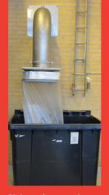
Discharge of compressed screen materials into Longofil bags which are well-suited as disposal bags for screen material.
