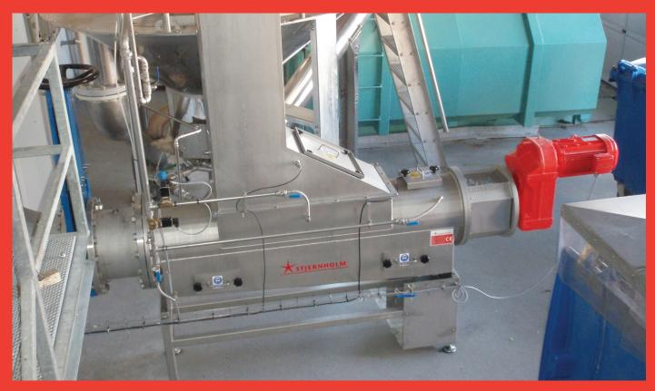
The Screenings Washing Press from Stjernholm is made of strong materials, is extremely hard-wearing and offers a verified long service life. In addition, Stjernholm AIS offers extra operational guarantees. The strong screw conveyor is made of steel quality S35J2G3 to ensure efficient transport and compression. In the washing section, technical water is used to remove remaining organic matter.
