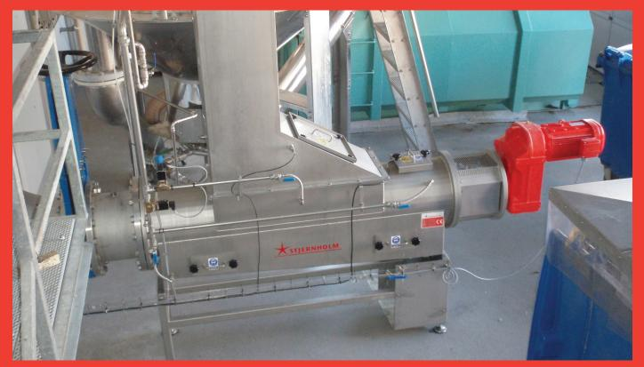
The Screenings Washing Press from Stjernholm is made of strong materials, is extremely hard-wearing and offers a verified long service life. In addition, Stjernholm AIS offers extra operational guarantees. The strong screw conveyor is made of steel quality S35J2G3 to ensure efficient transport and compression. In the washing section, technical water is used to remove remaining organic matter.
