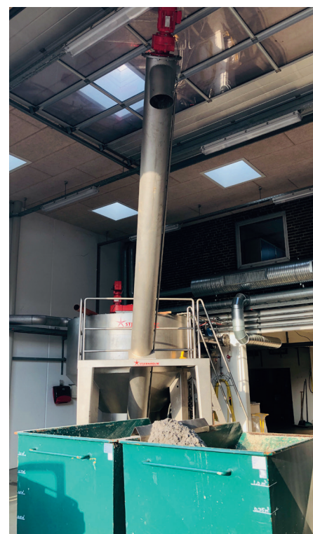
The washed sand is dried by gravity while conveyed directly to a container – ready for transportation and reuse.
