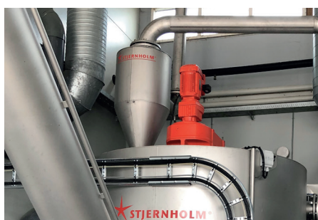
Capacity of the sand washer can be increased by mounting a cyclone at the inlet.
