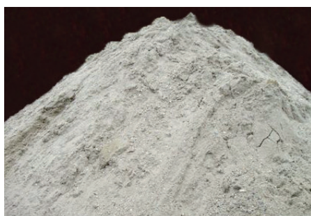
The sand final output contains less than 3% organics and 5% water.
