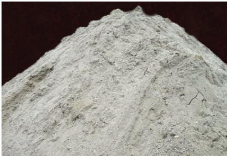
The grit final output contains less than 3% organics and 5% water.
