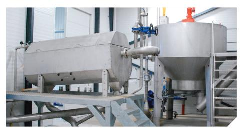
The system provides you; recycling of sand, reducing your purchase of sand by 92% - sand-free manure for easy application or use for biogas - separation of manure in a closed system which reduces emissions - a good investment.
