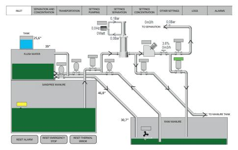
The system's flow is controlled by a flow and dry matter meter, which helps ensure the right balance between capacity and degree of separation.
