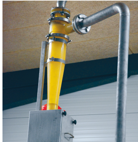
The separation of sand and organic matter takes place in the cyclone.
