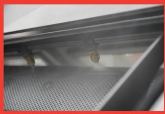
Flush water and brush are located towards the top of the drum. The flush nozzles and the brush are available in various sizes, types and qualities, and they are selected based on task and medium
