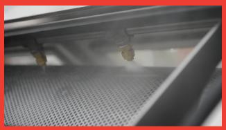
Flush water and brush are located towards the top of the drum. The flush nozzles and the brush are available in various sizes, types and qualities, and they are selected based on task and medium.
