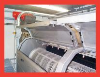
The drum, which rotates on 2 wheels and a bearing is driven by a gear motor. The drum can be driven by a frequency converter that ensures an optimal rotation speed.
