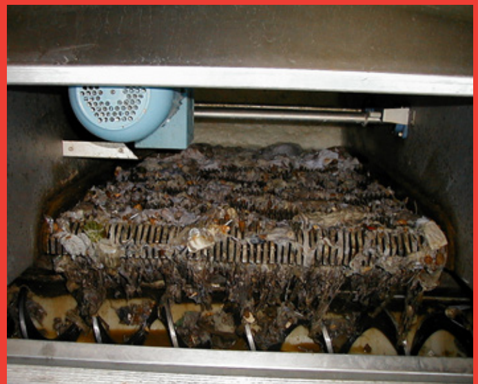
Installed with parallel screen bars where every second bar is moveable.
