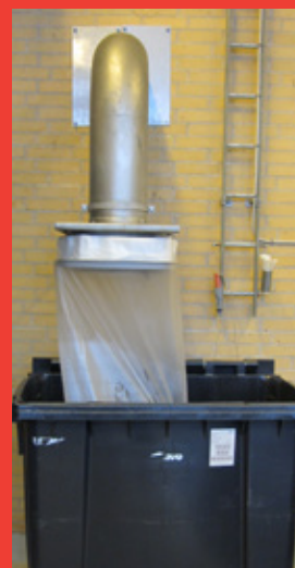
Discharge of compressed screen materials into Longofil bags which are well-suited as disposal bags for screen material. Continuous liner of plastic bags.
