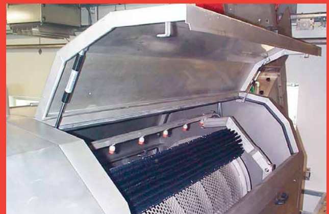
The drum is equipped with extra large hatches that facilitate easy inspection and service tasks. This ensures optimal working conditions for the operational staff.
