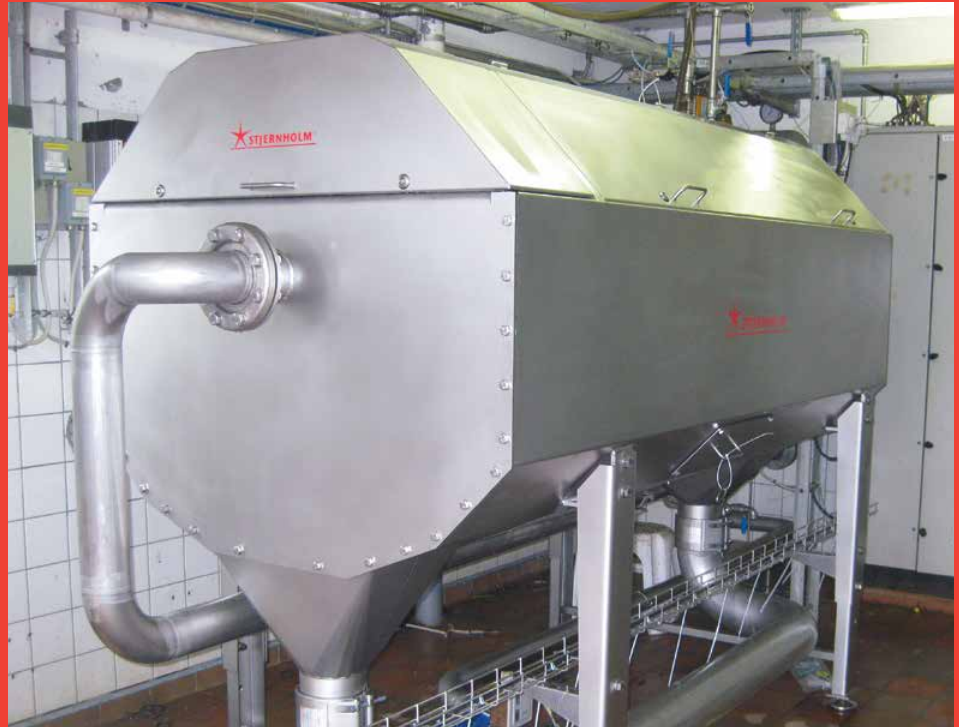
Drum Thickener / Drum Filter from Stjernholm are made of strong materials. They are particularly durable and designed for continuous use with a documented long service life.
