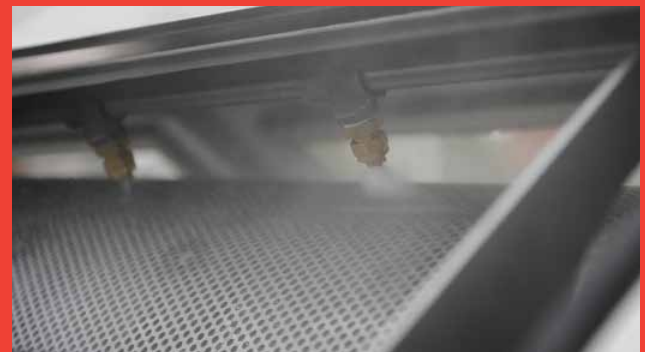
Flush water and brush are located towards the top of the drum. The flush nozzles and the brush are available in various sizes, types and qualities, and they are selected based on task and medium.
