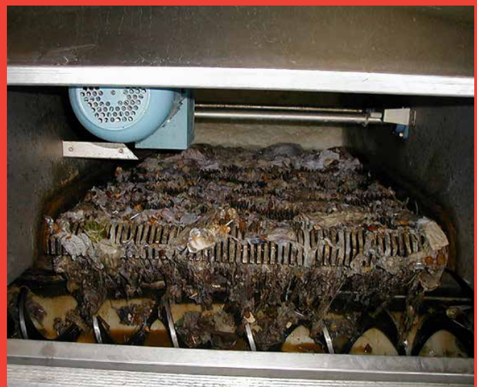
The Mechanical Fine Screen from Stjernholm features a solid construction and is run by a low-energy engine through a worm gear and a driving gear. The parallel screen bars, which are alternately fixated and moveable, ensure minimal crack openings in all operational situations.
