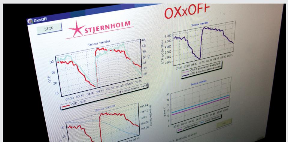
The historic data of the facility are collected on the memory card and can be used for Optimal control of aeration. Savings of up to 25 % of the energy consumption for bottom Aeration are easily obtained.
