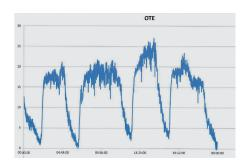
The image shows a measurement from the OXxOFF of the OTE (Oxygen Transfer Efficiency), before bottom and aeration blowers are connected with measurements from the OXxOFF. Major fluctuations in the OTE may be seen.
