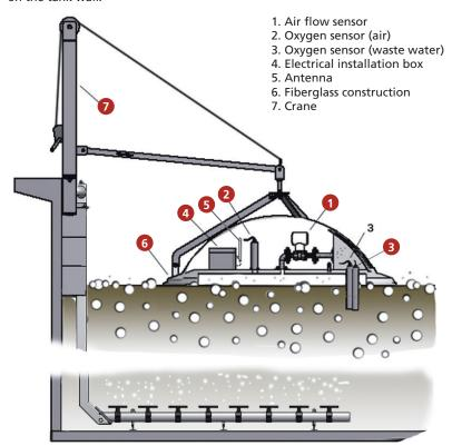
Stjernholm OXxOFF delivers a proven reduction of up to 25 % of the energy consumption for bottom aeration without any reduction of the effect
