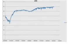
The image shows a measurement after the bottom aeration blowers have been controlled following measurements from the OXx-OFF. A significantly more stable and higher OTE can be seen which resulted in energy conservation for aeration of 20-25 %.
