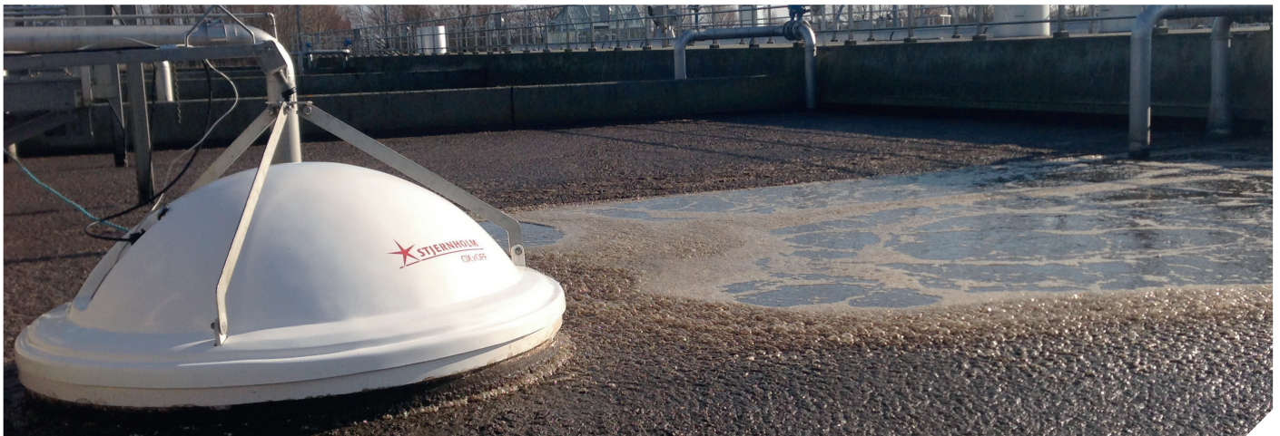
The OXxOFF has been developed with a unique programme that makes it possible to get immediate values for the oxygen transfer efficiency, (OTE), standard oxygen transfer efficiency (SOTE), oxygen transfer rate (OTR) and airflow.
