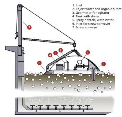
Stjernholm OXxOFF delivers a proven reduction of up to 25 % of the energy consumption for bottom aeration without any reduction of the effect
