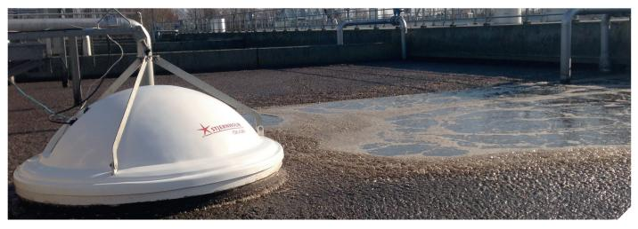
The OXxOFF has been developed with a unique programme that makes it possible to get immediate values for the oxygen transfer efficiency, (OTE), standard oxygen transfer efficiency (SOTE), oxygen transfer rate (OTR) and airflow.
