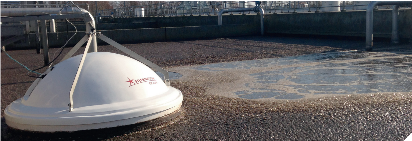
The OXxOFF has been developed with a unique programme that makes it possible to get immediate values for the oxygen transfer efficiency, (OTE), standard oxygen transfer efficiency (SOTE), oxygen transfer rate (OTR) and airflow.
