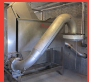
The compression pipe is shaped to ensure optimal transport of compressed screen material to the container.
