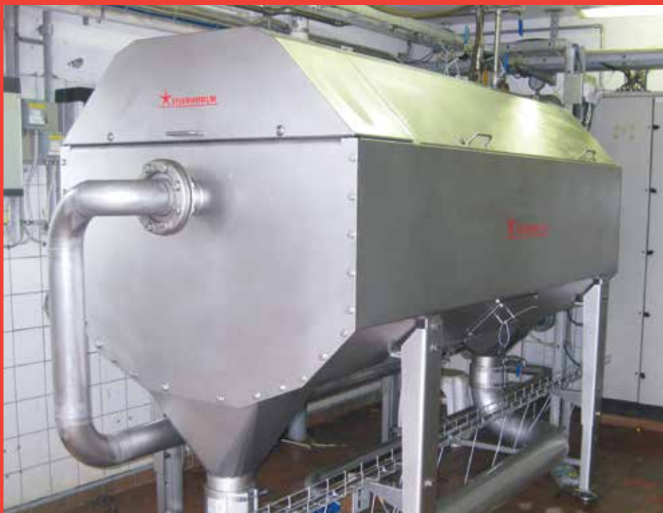
Drum Thickener / Drum Filter from Stjernholm are made of strong materials. They are particularly durable and designed for continuous use with a documented long service life.
