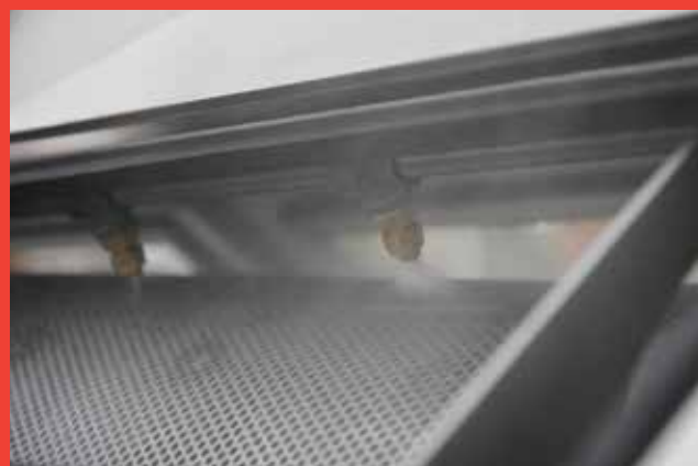
Flush water and brush are located towards the top of the drum. The flush nozzles and the brush are available in various sizes, types and qualities, and they are selected based on task and medium.
