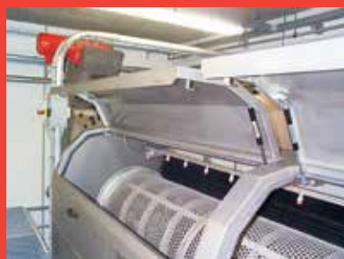
The drum, which rotates on 2 wheels and a bearing is driven by a gear motor. The drum can be driven by a frequency converter that ensures an optimal rotation speed.
