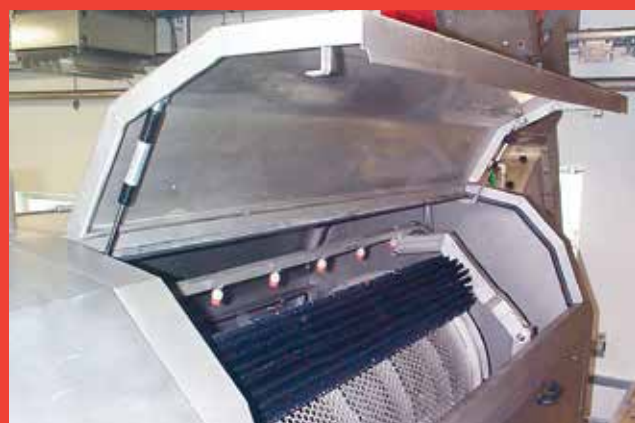
The drum is equipped with extra large hatches that facilitate easy inspection and service tasks. This ensures optimal working conditions for the operational staff.
